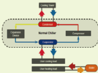
Traditional water-cooled chiller plus boiler
