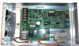
Modbus® Interface TCB-IFMB641TLE
